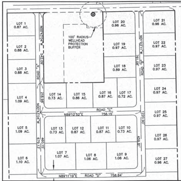
ROAD CENTERLINE BEARINGS AND DISTANCES 1"=200'
